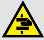
! There is a potential risk of trapping your fingers between the internal transmissions of the gears under the steering wheel. When the movement is directly carried out by the operator.
