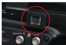
This Ethernet connector provides robust and fast connection to the network. It can be utilized for file transfer, live streaming, and camera control from a web browser.
