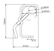
Work on diameters from 30mm to 52mm. The double locking knob position always provides an optimal grip point.
