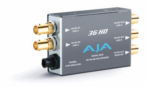
The 3GM is versatile and economical tool for interconnecting dual-link 1.5G SMPTE372M and 3G SMPTE425M. 3GM is bi-directional - allowing dual 1.5G to 3G or 3G to dual 1.5G conversion. Additionally, 3GM's 3G HD-SDI output is configurable for SMPTE425M type A or B. The 3GM can even convert 3G from/to type A or B. 3GM also provides a monitor output which is a single link SMPTE292M 1.5G HD-SDI. The 3GM is also compatible with SMPTE259M 270Mb SDI.
