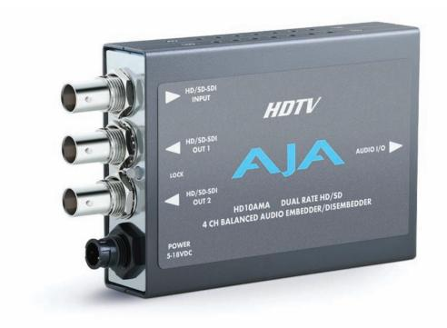
The HD10AMA is a dual rate 4 channel analog audio Embedder/Disembedder. The Disembedder is always functional providing 4 outputs. The Embedder is user selectable, on a channel pair basis, to either "pass" input audio or embed input audio from the breakout cable. Analog audio levels are selectable. The HD10AMA automatically detects and configures to the input video standard. 8 x XLR breakout cable included.
