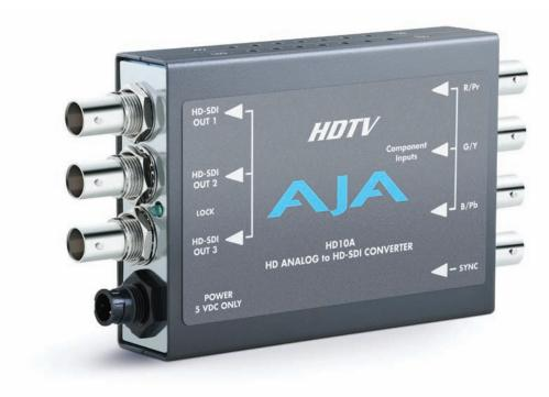
The HD10A is a miniature, high-quality, 10-bit analog to digital converter for HDTV. A companion to the popular HD10C2 D/A converter, the HD10A can add an HD-SDI output to cameras, computers with HD RGB, VTRs, or other analog-only high definition equipment. The HD10A accepts RGB or YPbPr analog HD and outputs three duplicate HD-SDI signals. Works in 1080/1035i and 720p with internal or external sync (tri-level).
