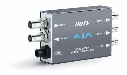
The HD5DA is a miniature, low-cost 1x4 HD/SD-SDI distribution amplifier/repeater. Featuring four separately buffered HD/SD-SDI outputs, the HD5DA provides automatic HD cable equalization to 125 meters and automatically adapts to 143, 177, 270, 360 Mb, and 1.5Gb SDI.
