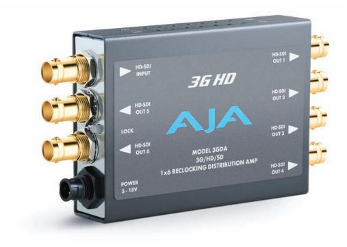
The 3GDA is a miniature, low-cost 1x6 3G/HD/SD-SDI input, re-clocking distribution amplifier. Featuring six separately buffered SDI outputs, the 3GDA provides automatic input detection, re-clocking and cable equalization.
