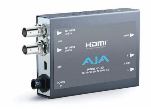
The Hi5-3G converts 3G-SDI, dual or single link HD-SDI, or SD-SDI to HDMI v1.3a for driving HDMI monitors. HDMI v1.3a capability at 30 bits per pixel allows full support of the latest 10 bit monitors. Audio is supported in the HDMI output allowing a convenient single cable audio/video connection. The Hi5-3G provides 2 Channel RCA style audio outputs for separate audio monitoring if needed. USB connectivity allows for easy PC/Mac setup and field upgrades.
