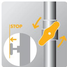
Captive handle: thanks to this special machining on the threads, it is impossible to loose the handle even if completely unscrewed.
