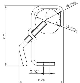
Work on diameters from 30mm to 52mm. The double locking knob position always provides an optimal grip point.
