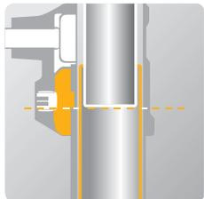
Captive collars: thanks to a special design, even if the user unscrews the locking nut, of this component the inner alu insert and dedicated machining of the tube does not allow for the column to separate.
