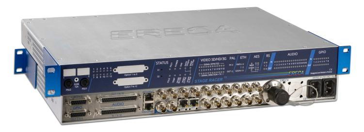
The STAGE RACER is a complete optical fiber transmission solution for Outside Broadcast events, OB trucks, Commentary positions, Stage-Studio connection and Building Infrastructure.
