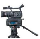
Connect Ki Pro to a wide variety of professional HD cameras via component or HD-SDI. The Apple ProRes 422 recordings that Ki Pro produces rival the native recordings of many HD cameras. Apple ProRes 422 recordings are full raster video at 10-bit quality whereas typical camera recordings produce a variety of compressions, horizontal resolutions, file types, and are often only at 8-bit.
