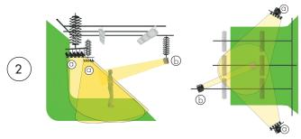
Placing whole banks of parallel dedolights on both sides (29), controlling each bank of the lights in an identical way by DMX control, the actor can be lit from the knee upward without causing any noticeable shadows on the green floor. Even if the dedolights are placed in such a way that they are looking downward at a moderate angle, the shadows can be projected to fall outside of the 'action area'.
