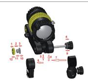
Hot shoe mount can be exchanged by the user to stand fitting and vice versa, as shown above.
