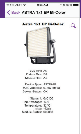
System information for a single fixture
