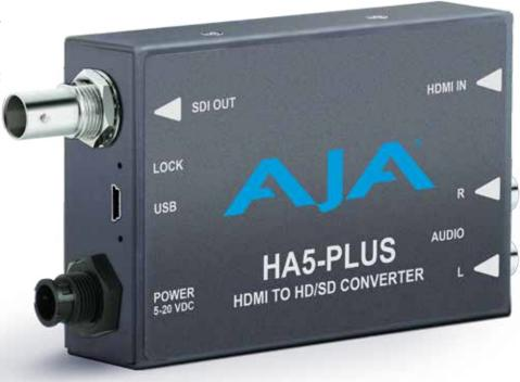
HA5-Plus is AJA's next generation HDMI-to-SDI Mini-Converter. The HDMI input is converted to SD, HD, or 3G-SDI, depending on the input format, for driving SDI equipment. Up to eight channels of HDMI audio are embedded into the SDI output and a 2-channel RCA analog input allows embedding of separate audio into the SDI output, all user configurable. The HA5-Plus also accepts progressive SD (480p, 576p) for compatibility with many DSLR cameras.
