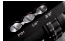
Parking position for spare camera screws
