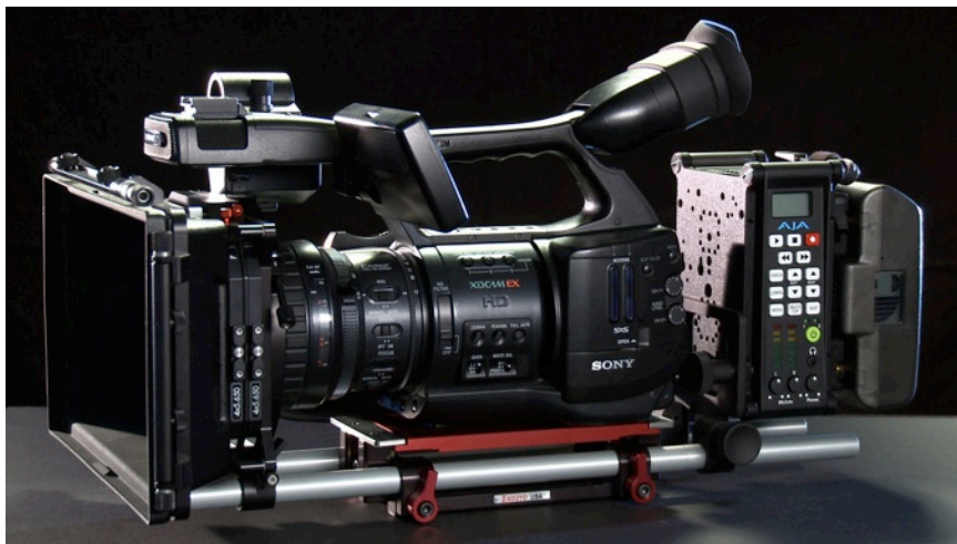
Ki Pro Mini with two Mini Mount Plates for attachment to camera and 3rd Party device attachment
