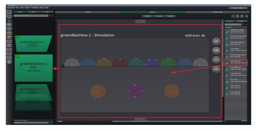
Above the constellation list, you will find the "Deploy" button (see red rectangle in image below). Once you have dropped the constellation onto a greenMachine, the "Deploy" button will be highlighted in two possible colors:
