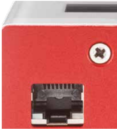
All miniCASTER® top shot showing the Ethernet RJ45 port for landline connections
