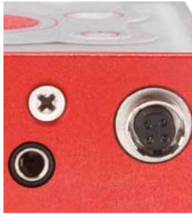
miniCASTER® analog-bottom shot showing the composite/ audio-in mini-jack and moxex locking power connector
