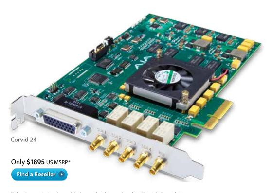
Take the next step in multi-channel video and audio I/O with Corvid 24. Supporting up to 4 independent\* channels of capture or output with separate LTC, embedded 24-bit audio and metadata for each channel all on a single PCIe card, Corvid 24 is the solution for high-density I/O. All four connections can also be used to support full 4K I/O. The choice is yours. And with multiple operating system support, Corvid 24 will work in almost any environment.
