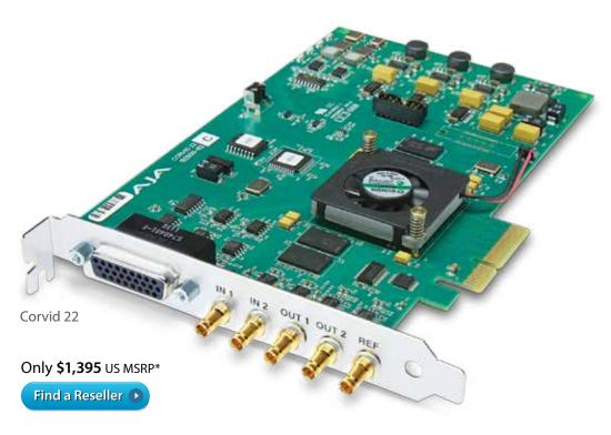
Get multiple I/O channels without taking up a lot of space. Corvid 22 provides high-performance, dual-channel video and embedded 24-bit audio I/O in a single PCIe card. Two completely independent channels handle resolutions up to 2K and high-framerate 3G as well. With separate LTC and RS-422 machine control per channel and support for multiple operating systems, Corvid 22 gives you all the performance and capabilities you need.
