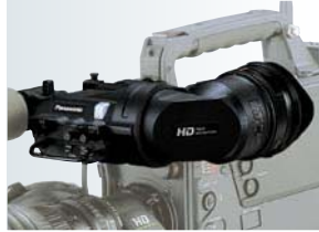
AJ-HVF21KG 50.8 mm (2 inches) HD EVF 59.94 Hz/50 Hz Switchable Not available in some areas.
