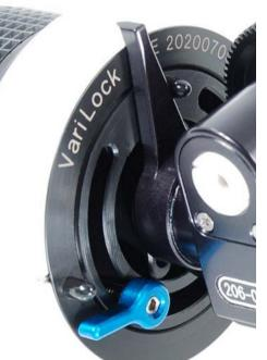
The VariLock® feature of the Rigs now allows both, since the range of rotation is fully variable for any selectable limit.
