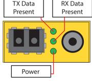
WARNING: Module laser is active as soon as power is connected, regardless of LED indication
